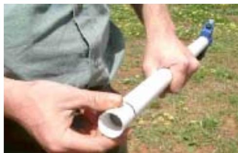
2. Remove the lid of the *top cap* and extract the probe electronics. Place this safely to one side on a clean, dry surface such as a tarpaulin.
