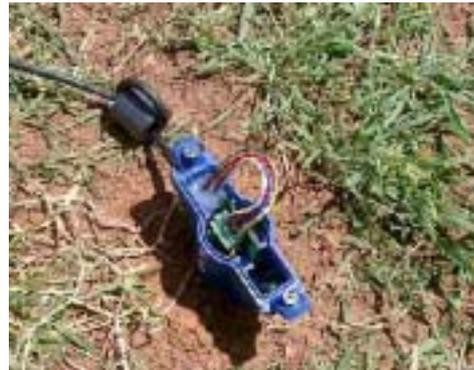
3. Ensure that the sealing gasket on the top cap is **clean**, in **good condition** and positioned correctly, and replace the *lid* of the *top cap*. Tighten the screws evenly completely to ensure an effective seal.
