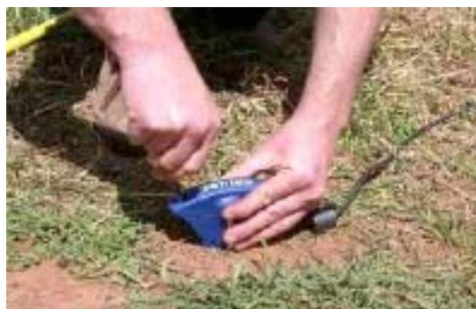
4. Tighten the *FairRite bead* into position and tighten the cable gland. The probe is now installed and upon connection to the data logger is ready for use.
