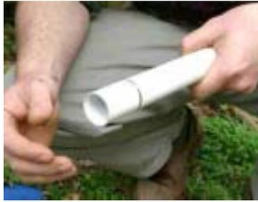
2. Remove the lid of the *top cap* and extract the electronics. Place this safely to one side on a clean, dry surface such as a tarpaulin.
