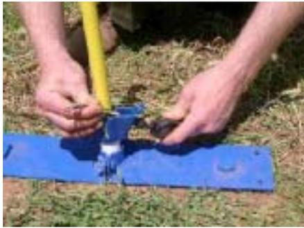
6. Remove the *stabilization plate wing nuts*.
