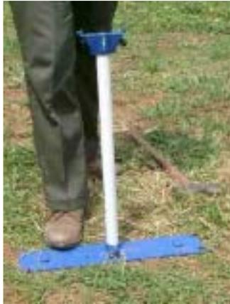
2. As the probe enters the prepared hole in the soil, it shaves off a soil residue that is eventually stored in the cutting tip or falls to the bottom of the hole.
