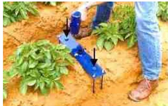
11. The *stabilization plate* should be firm to the ground without causing significant soil compression
