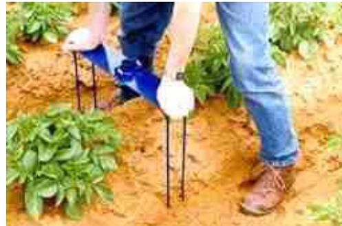
10. Using a *sledgehammer* alternately beat the *stabilization plate* at the points provided to force it closer to the ground. Do not beat continuously on any one side in advance of the other. The aim is to achieve a situation where the pins are near parallel in the ground.
