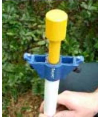
5. Continue inserting the *probe* by hammering on the insertion dolly with a *sledgehammer* until there is a 2.5 cm (1 inch) gap between the base of the *top cap* and the edge of the *stabilization plate* tube guide.
