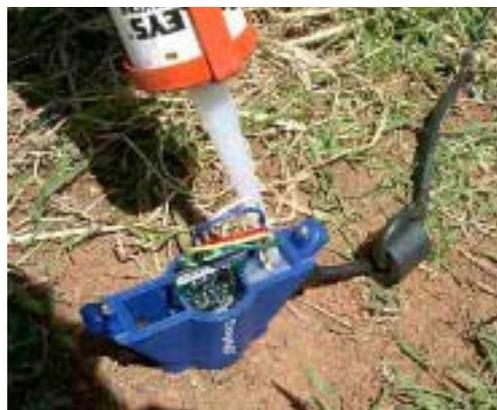
3. Ensure that the sealing gasket on the top cap is **clean**, in **good condition** and positioned correctly, and replace the *lid* of the *top cap*. Tighten the screws evenly completely to ensure an effective seal.
