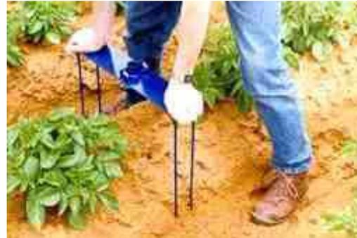
4. Using a *sledgehammer* alternately beat the *stabilization plate* at the points provided to force it closer to the ground. Do not beat continuously on any one side in advance of the other. The aim is to achieve a situation where the pins are near parallel in the ground.
