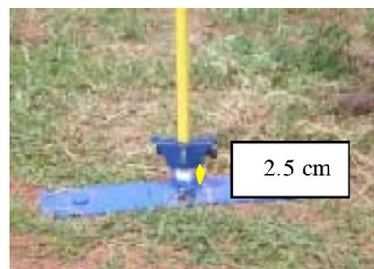
**Note:** This clearance height is important. If you hammer the probe in too far you will not be able to lift the stabilization plate off the long stabilization plate pins.
