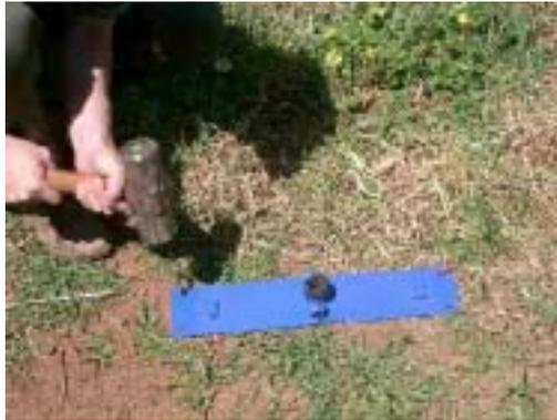
3. Drive the *stabilization plate pins* all the way into the ground using a *sledgehammer*. The *stabilization plate* should be in firm contact with the soil without compressing it significantly.
