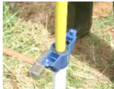
4. Continue inserting the *probe* by hammering on the insertion dolly with a *sledgehammer* until there is a 2.5 cm (1 inch) gap between the base of the *top cap* and the edge of the *stabilization plate* tube guide.
