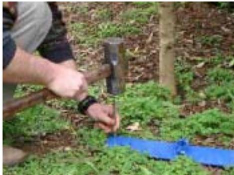
4. Put the soil sampler *polyguide* in place. The *stabilization plate* is now ready for insertion of the *AMS soil sampler*.
