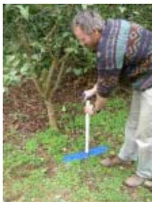
3. As the probe enters the prepared hole in the soil, it shaves off a soil residue that is eventually stored in the cutting tip and at the base of the hole.
