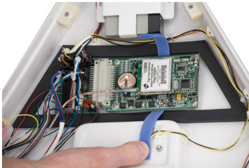
FIGURE 6-11. Removing the Velcro strap
