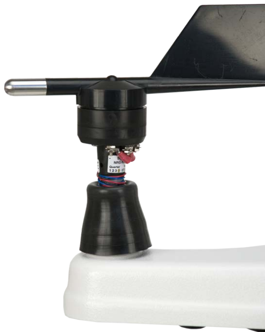
FIGURE 6-7. Wind direction sensor with boot down and exposing wires
