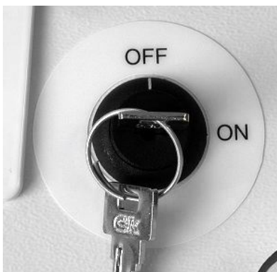
FIGURE 4-3. Keyed power switch is located on the bottom of the TurfWeather
