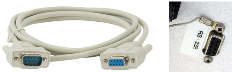
FIGURE 4-2. Serial cable (left) and the weather station serial port in which the serial cable male connector connects
