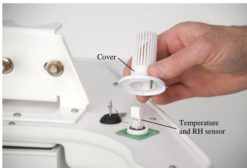
FIGURE 6-3. Removing the temperature and RH sensor cover
