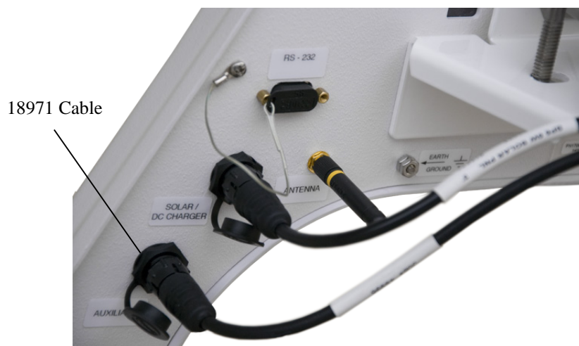
FIGURE 5-22. 18971 cable connected to TurfWeather station
