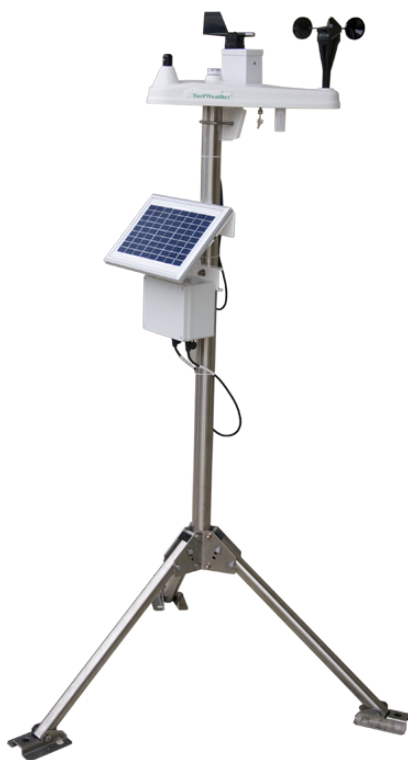
FIGURE 5-16. Short haul enclosure mounted to the 16776 tripod
