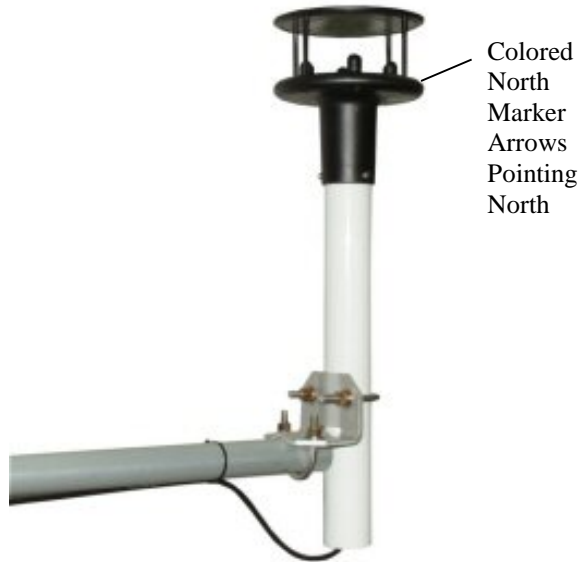
FIGURE 7-1. WindSonic mounted on a CM202 using pn 17837
