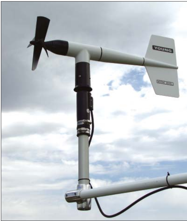
This 05106 Wind Monitor-MA is attached to a crossarm via a 17953 NU-RAIL fitting and a mounting pipe (shipped with the sensor).
