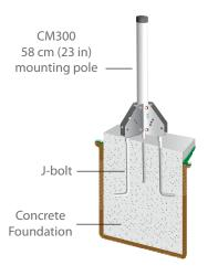
A cut away view shows a 58 cm (23 in) pole attached to a concrete foundation via j-bolts. Order a CM300-PJ to get a 58 cm (23 in) pole with the J-bolt pedestal kit.
