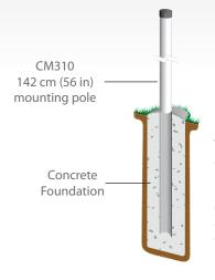
This cut away view shows a 142 cm (56 in) mounting pole placed directly in a concrete foundation. Order a CM310-NP to get a 142 cm (56 in) pole without a pedestal kit.
