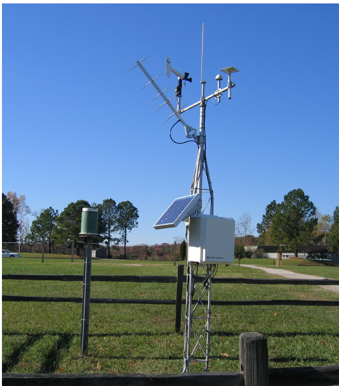
This station for the National Estuarine Research Reserve (NERR) in Virginia transmits data using a satellite transmitter.
