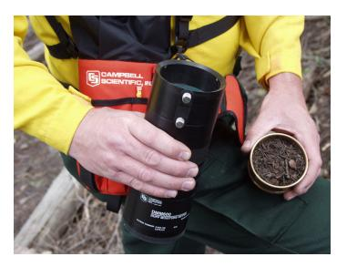
To measure duff water content, the sample is placed in the sample chamber and the compression knob is turned until an audible indicator signals the sample is properly compressed and the measurement is complete. download and upload calibration coefficients, monitor the battery voltage, and reset the DMM600.
