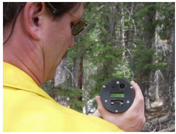
Total time for measurement is about 30 seconds. Measurements derived from the standard and user-defined calibrations are alternately displayed on the LCD if a user-defined calibration has been downloaded.
