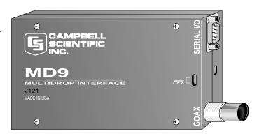
The network is accessed through the computer's serial port. LoggerNet Datalogger Support Software supports station addressing, data retrieval, and monitoring. Remote MD9 networks are accessed by telephone (see page 3) or radio telemetry (contact Campbell Scientific).
