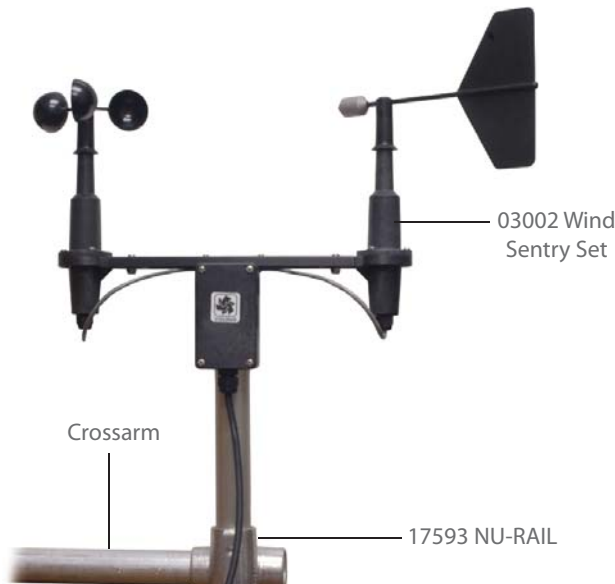
Wind sets are attached to CM200-series crossarms either using a NU-RAIL fitting (shown above) or the CM220 mounting bracket (shown below).
