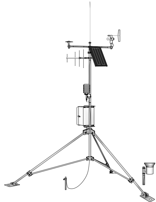
A remote meteorological station can transmit data via radio telemetry to a base station.
