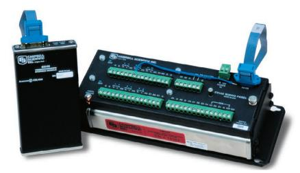
A CR10X sends historical or real-time data to an SM4M. Data can be sent automatically to a connected module or manually initiated with a keyboard display.
