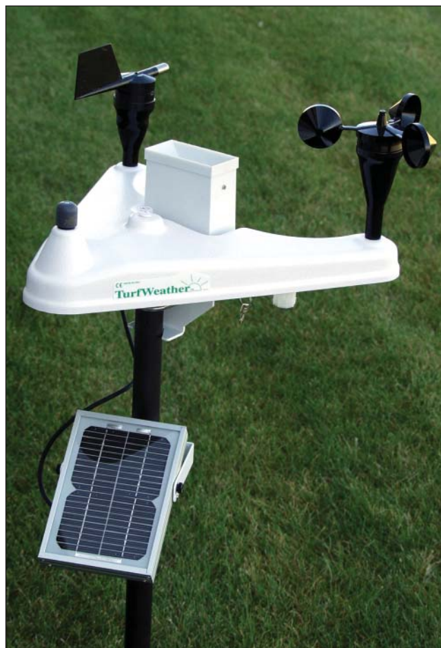
TurfWeather can provide real-time weather measurements and calculate ETo on an hourly and daily basis.
