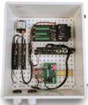
ESS Remote Processing Unit
