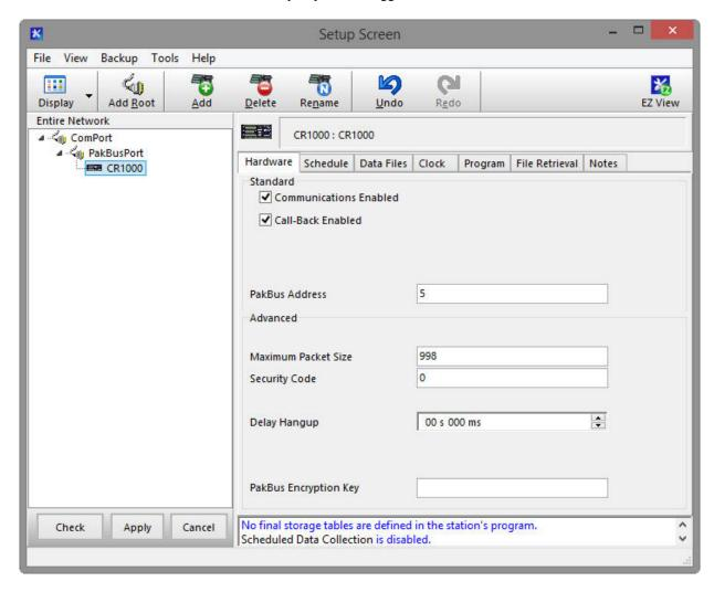
Press the **Apply** button to save your changes. You are now ready to connect to your datalogger using the *LoggerNet Connect* screen.
