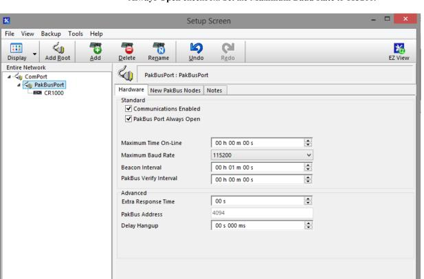
Select the **PakBusPort** element in the tree, and select the **PakBus Port Always Open** checkbox. Set the **Maximum Baud Rate** to **115200**.
