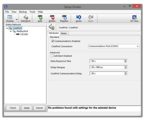
With the setup tree entered, you will now need to complete the configuration of each element. Start with selecting the **ComPort** element at the root of the tree. Under **ComPort Connection**, select port labeled **RF407-Series**.
