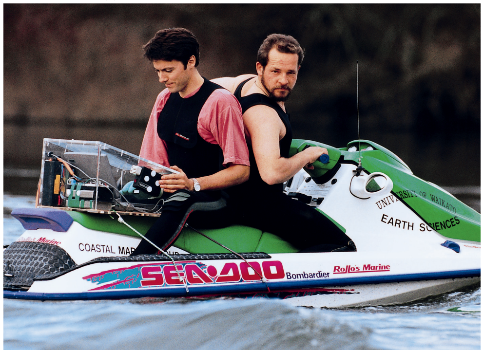
The University of Waikato's Seadoo-based system measures and records water depth versus geographic position, making the system ideal for surf-zone bathymetry. (Photo courtesy of the Waikato Times, NZ)
