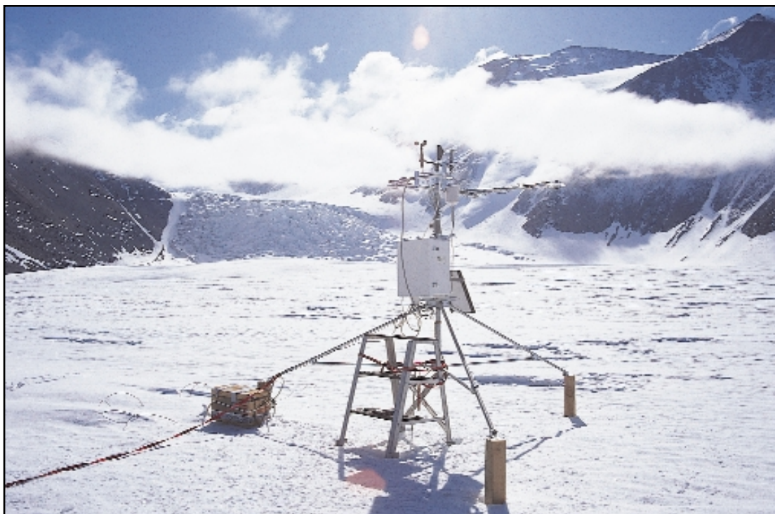
Eddy correlation station provides data for energy balance studies. (Canada Glacier, Taylor Valley, Antarctica).
