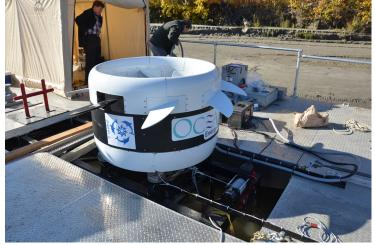
of hydrofoils that extend radially inward and outward from the annulus-shaped rotor. The mating annular stator includes a patented nine-phase electrical generator and permanent-magnet bearings.
