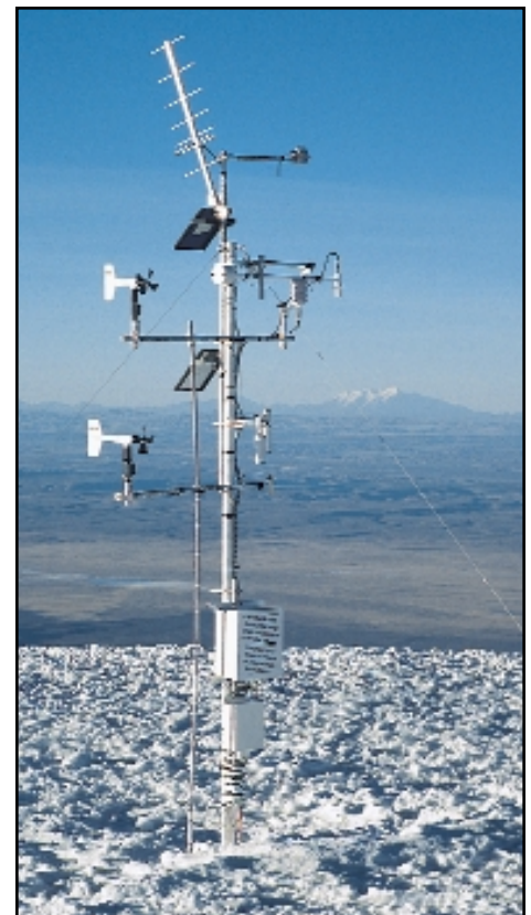
The Nevado Sajama weather station measures a variety of meteorological and snow parameters, many redundantly, to ensure data capture and integrity.
