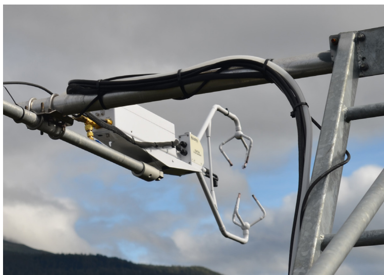
The CPEC200 with vortex intake at the top of the 80-m Warra flux tower
