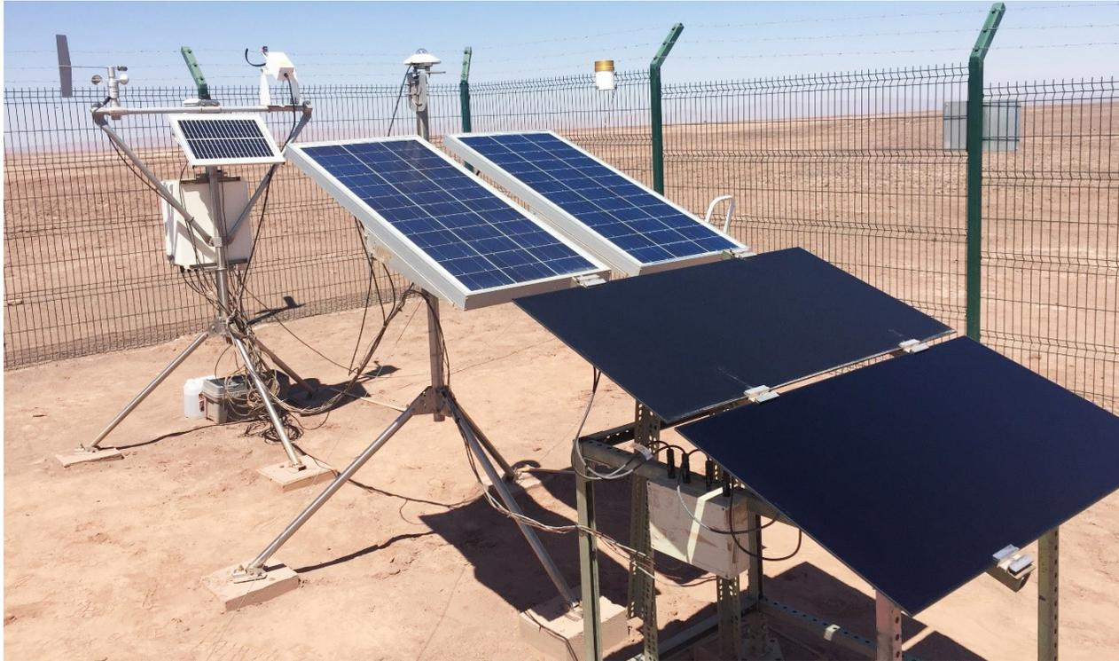
Valhalla, an energy company in Chile, is making resource assessment and solar-panel soiling measurements in advance of construction of the Cielos de Tarapacá Project.
