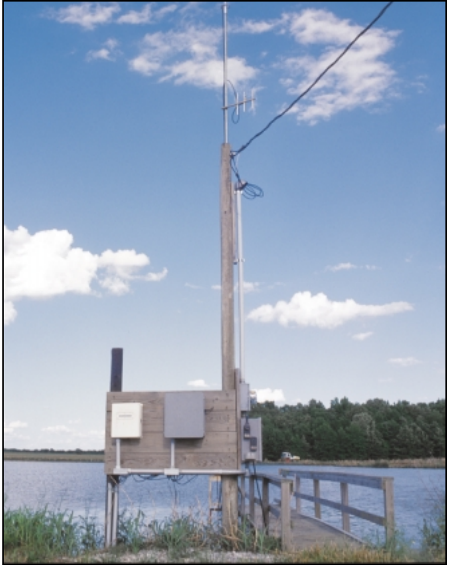
A Campbell Scientific CR10 Monitoring and Control system eliminates the need to manually check DO concentrations several times a night. Alarms are sent via RF to a computer.
