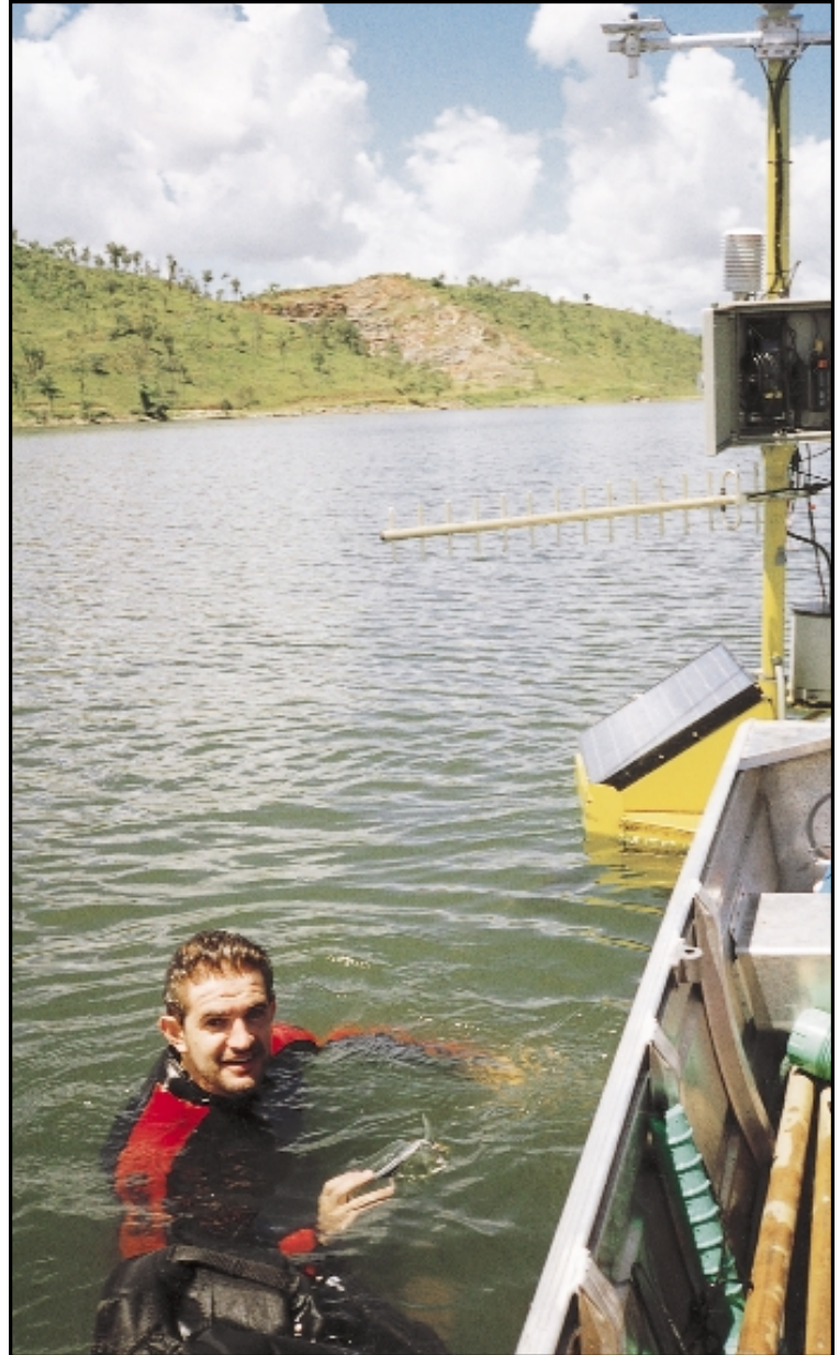
Campbell Scientific Australia's Chris Kellet installs the underwater thermistor chain on Ross River Dam's weather station.
