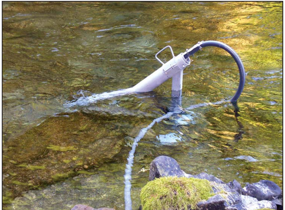
Above: A custom-built sensor stand holds the FTS DTS-12 turbidity sensor in the Cedar River.
