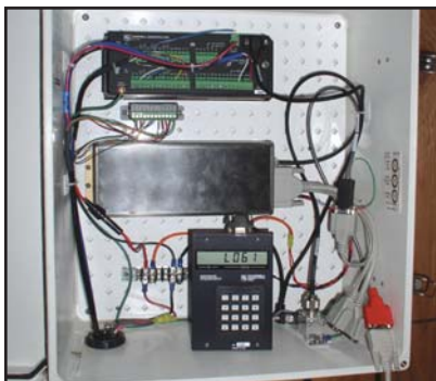
Instrument Enclosure with CR10X and MCC low-band radio.
