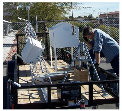
readied for transport in under an hour and be back in use within an hour of arrival at its next location. Other advantages of placing the equipment on a flat bed are that the equipment maintains the same configuration from location to location and has a relatively small footprint, and that equipment or instruments can be added or taken off as necessary.
