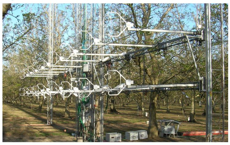
Campbell micromet sensors used in intensive turbulence array
