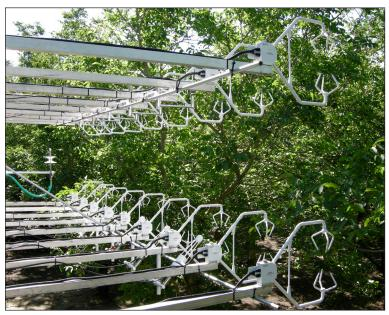
Anemometers, Campbell KH2O Krypton Hygrometers, carbon-dioxide sensors, and various other environmental sensors, all mounted at precise intervals on a horizontal frame. The CSAT3 provides precision, three-dimensional turbulence measurements, with a body and frame designed for minimal flow distortion.
