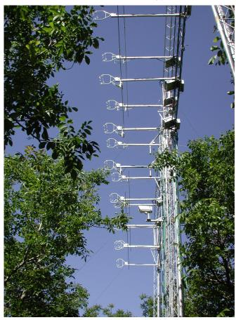
used to measure the same thing, providing comparative data for researchers. Also, the horizontal array could be raised and lowered to take measurements within and above the canopy.
