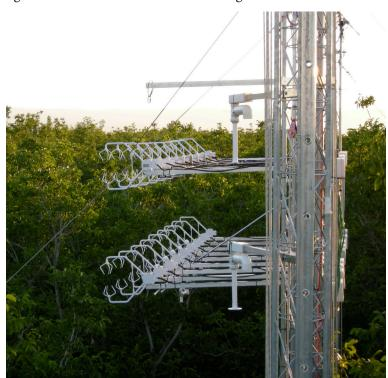
between small-scale and large-scale eddies in order to test and improve the sub-filter-scale closure models used in large-eddy simulation of turbulent flows. In addition to the horizontal array, for the CHATS project the researchers included a vertical array on a 30 m tower, using 13 CSAT3 anemometers, 6 KH2O hygrometers, and many other sensors.
