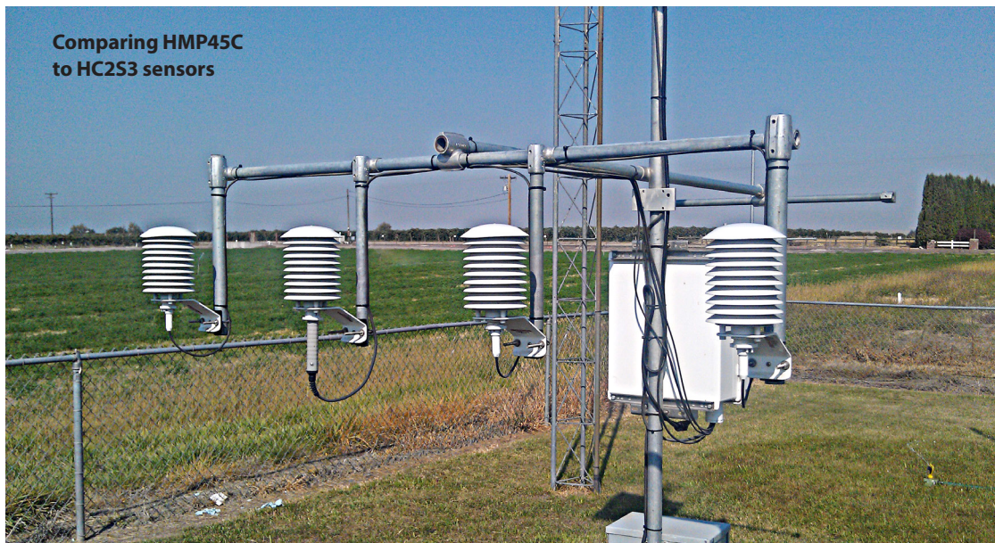
Comparison array testing 107-L temperature sensors
