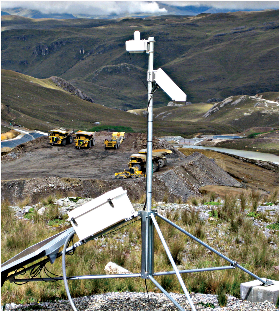
Warning system with CS110 Electric Field Meter
