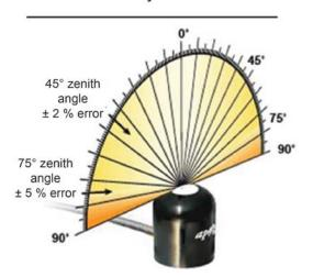
Directional, or cosine, response is defined as the measurement error at a specific angle of radiation incidence. Error for Apogee silicon-cell pyranometers is approximately  $\pm$  2 % and  $\pm$  5 % at solar zenith angles of 45° and 75°, respectively.
