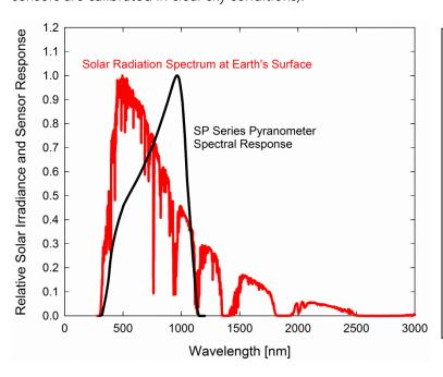
Spectral response of Apogee SP series pyranometers compared to solar radiation spectrum at Earth's surface. Silicon-cell pyranometers, such as Apogee SP series, are only sensitive to the wavelength range of approximately 350-1100 nm, and are not equally sensitive to all wavelengths within this range. As a result, when the spectral content of solar radiation is significantly different than the spectrum that silicon-cell pyranometers were calibrated to, spectral errors result.
