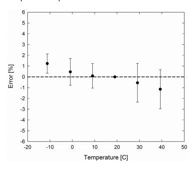
Mean temperature response of ten Apogee silicon-cell pyranometers (*errors* bars represent two standard deviations above and below mean).
