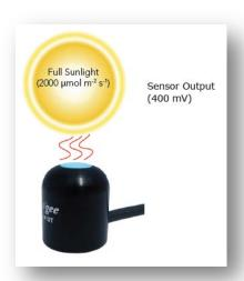
Example of PPF measurement with an Apogee quantum sensor. Full sunlight yields a PPF on a horizontal plane at the Earth's surface of approximately 2000  $\mu mol~m^{-2}~s^{-1}$ . This yields an output signal of 400 mV. The signal is converted to PPF by multiplying by the calibration factor of 5.00  $\mu mol~m^{-2}~s^{-1}$  per mV.
