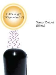
Example of UV measurement with an Apogee UV sensor. Full sunlight yields UV radiation on a horizontal plane at the Earth's surface of approximately 175  $\mu$ mol m<sup>-2</sup> s<sup>-1</sup>. This yields an output signal of 35 mV. The signal is converted to UV radiation by multiplying by the calibration factor of 5.0  $\mu$ mol m<sup>-2</sup> s<sup>-1</sup> per mV.
