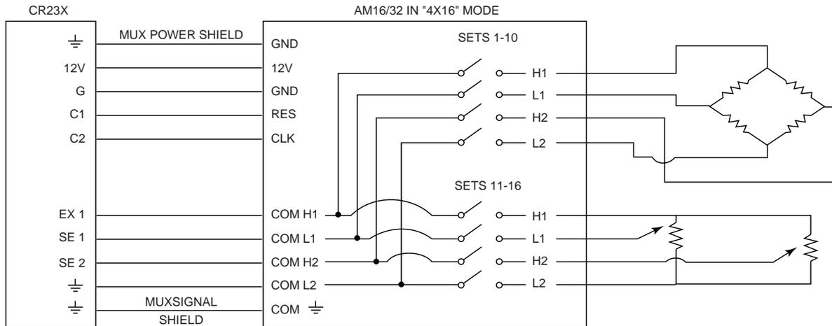
FIGURE 9. Wiring Diagram for Strain Gages and Potentiometers
