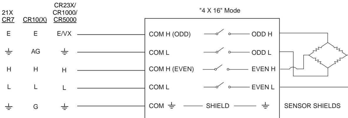
FIGURE 15. Full Bridge Measurement
