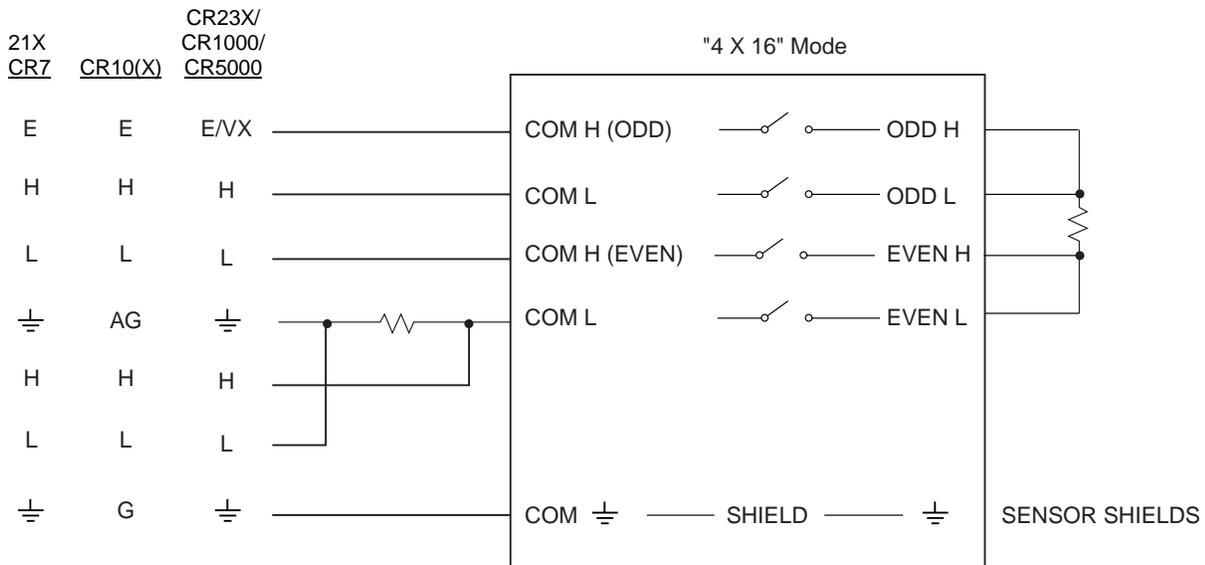
FIGURE 14. Four Wire Half Bridge Hook-up and Measurement
