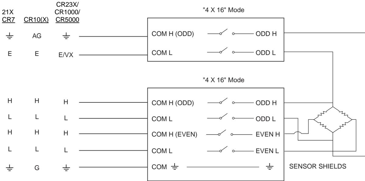
FIGURE 16. Full Bridge Measurement with Excitation Compensation
