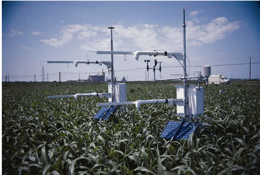
FIGURE 2-1. ASPTCs Mounted to Bowen Ratio Arms
