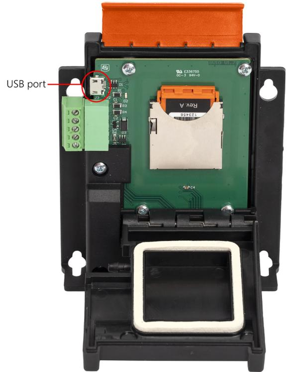
FIGURE 4-1. BaroVUE 10 with main door open
