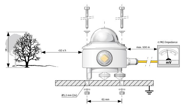
FIGURE 7-1. Pyranometer installation
