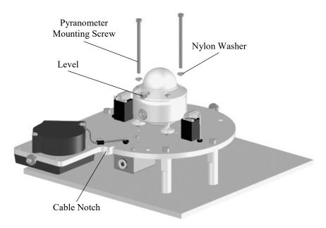
FIGURE C-7. Mounting the pyranometer to the CVF4
