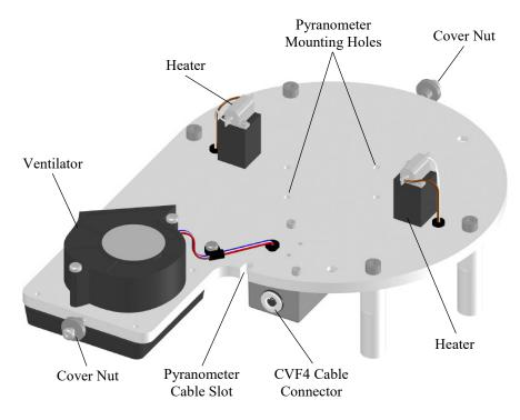
FIGURE C-1. CVF4 Components (top view, no cover)
