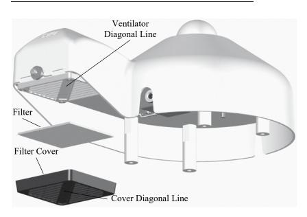
FIGURE C-11. CVF4 filter replacement
