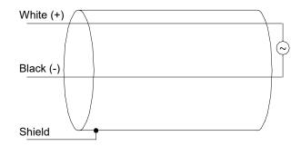
FIGURE 7-6. Thermopile detector schematic
