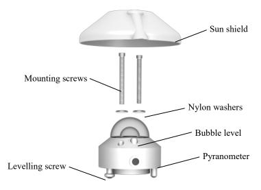
FIGURE 7-5. Exploded view of the pyranometer
