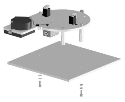
FIGURE C-6. Mounting CVF4 feet to a mounting stand
