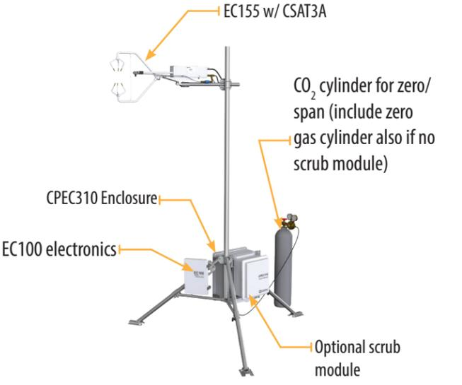
4. Connect the sensor head to the measurement electronics.
