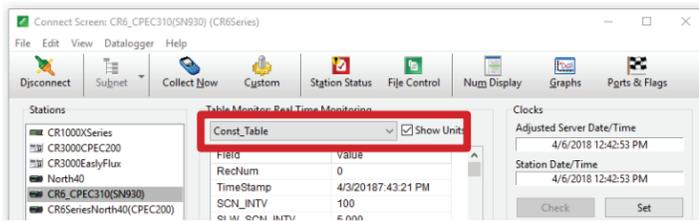
3. Set the variables listed below to enable auto zero and span. -1 indicates true and 0 indicates false. **ZRO\_SPN\_INVNT** is the number of days between zero and span and **ZRO\_SPN\_OFST** is the minutes after the auto zero and span begins
