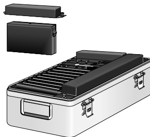
FIGURE 1.2-1. CR9000X battery pack
