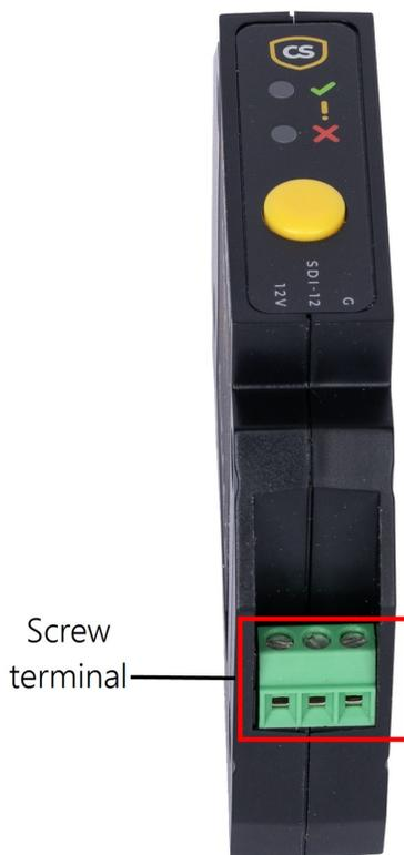
Figure 7-4. CS211 3-pin screw terminal
