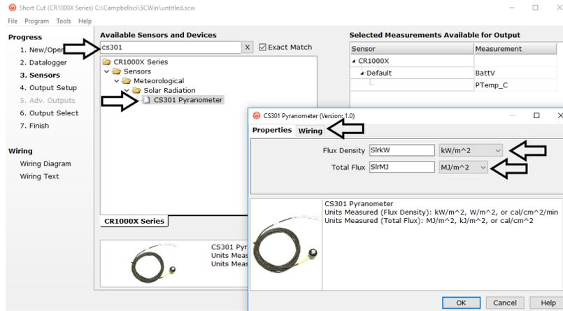
4. Click on the **Wiring** tab to see how the sensor is to be wired to the datalogger. Click **OK** after wiring the sensor.
