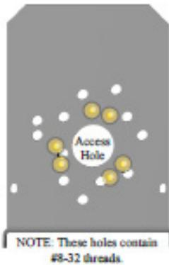
Mounting holes used for the CS300 and CS301 are indicated in yellow.
