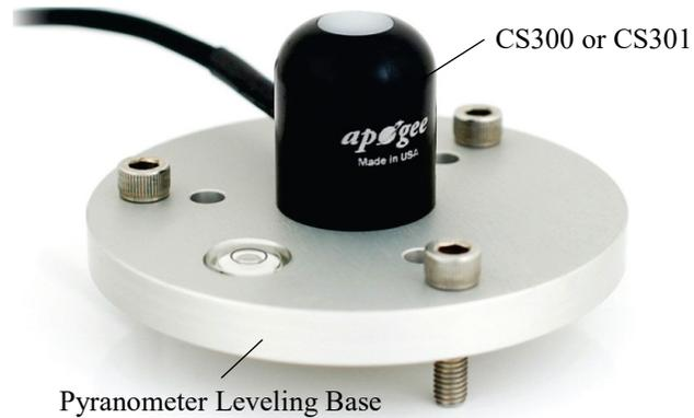
4. Loosely mount the pyranometer leveling base on the CM225 or 015ARM. Do not fully tighten the three mounting screws.
