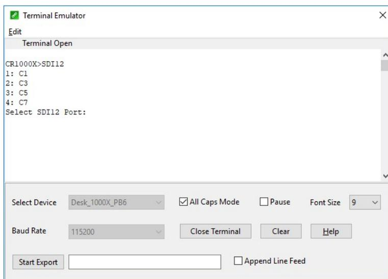
8. At the **Select SDI12 Port** prompt, type the number corresponding to the control port where the sensor is connected and press Enter. The response **Entering SDI12 Terminal** indicates that the sensor is ready to accept SDI-12 commands.
