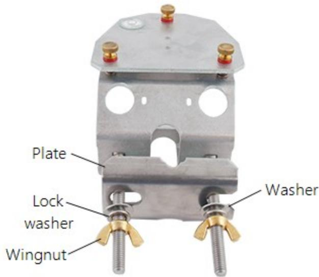
4. Place the vertical pipe or crossarm between the plate and bracket, then tighten the wing nuts until the lock washers are compressed.
