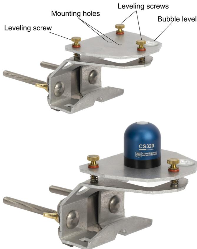
3. Place the screws, plate, washers, lock washers, and wing nuts in the side holes if using a vertical pipe or in the bottom holes if using a crossarm.
