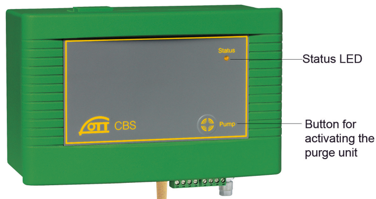
FIGURE 7-4. Purge Button and Status LED
