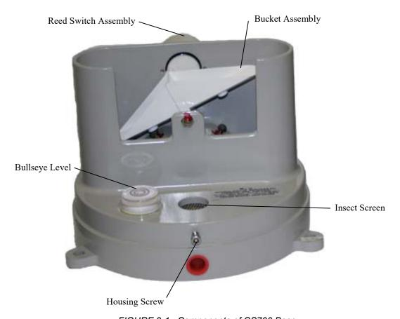
FIGURE 9-1. Components of CS700 Base
