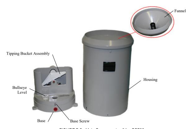
FIGURE 7-5. Main Components of the CS700
