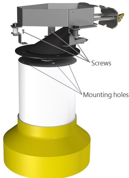
FIGURE 6-6. Mounting CM270 to the rain gage
