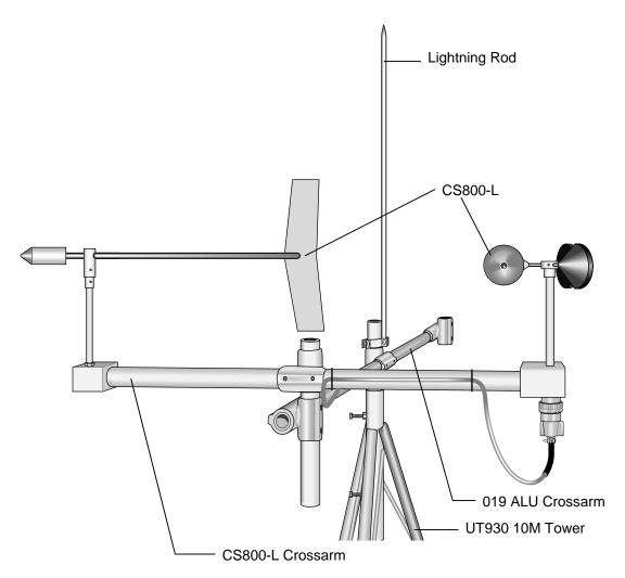
Figure 1. CS800-L Climatronics Wind Speed and Direction Sensor
