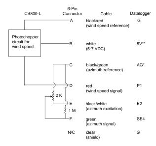
Figure 3. CS800-L Wiring
