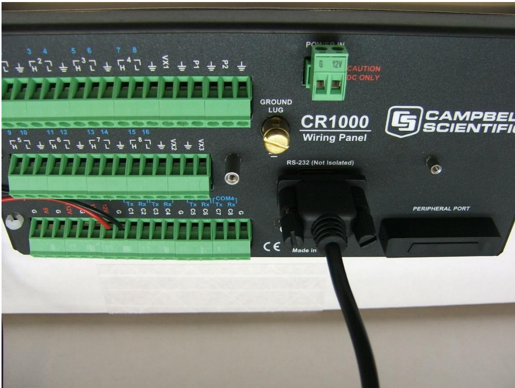
FIGURE 9-7. Modem connection to data logger RS232 port
