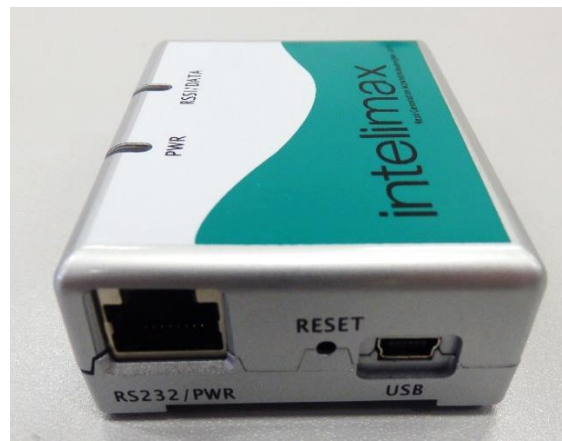
FIGURE 6-4. RJ45 socket, reset button and mini USB socket
