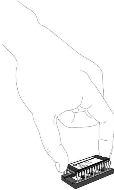
**FIGURE I-6. Inserting the New PROM**
