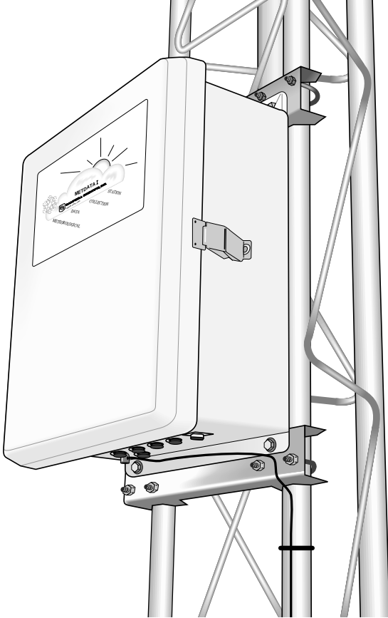
FIGURE 3.1-2. MetData1 Enclosure on UT10 or UT30 Tower
