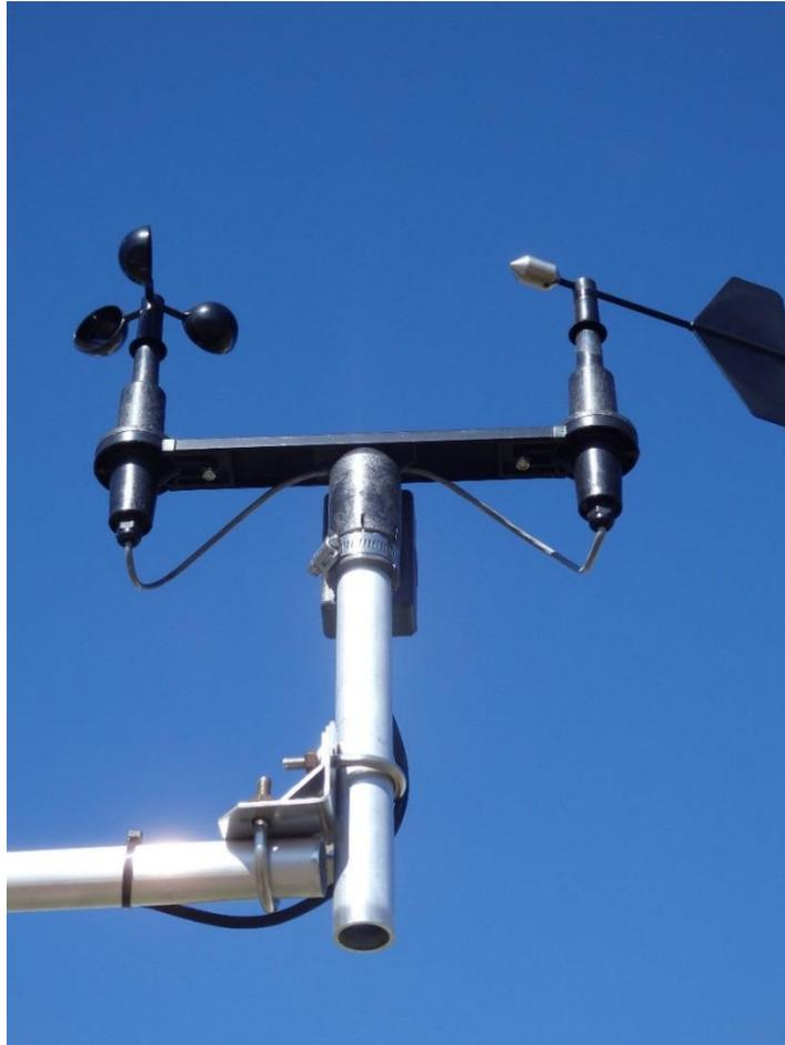
*FIGURE 3-7. Installed 03002 Wind Sentry*
