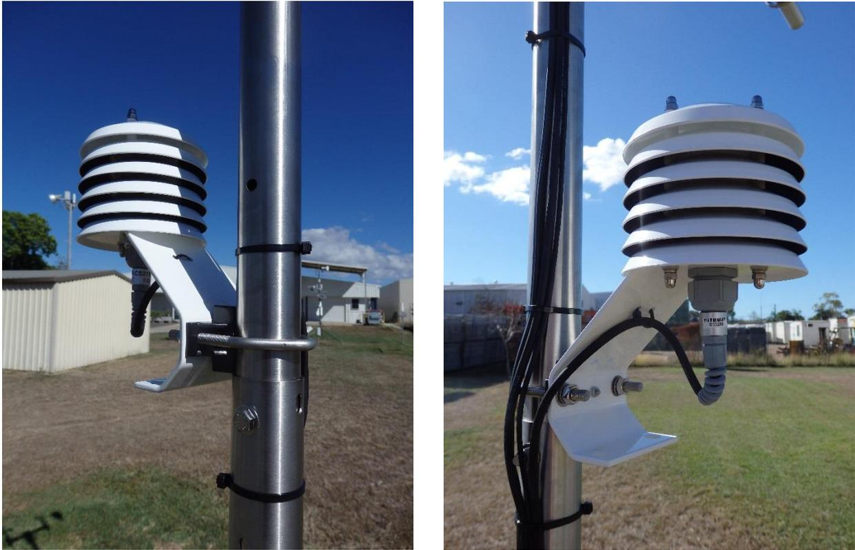
*FIGURE 3-4. CS215-MET2 mounted on a tripod mast*
