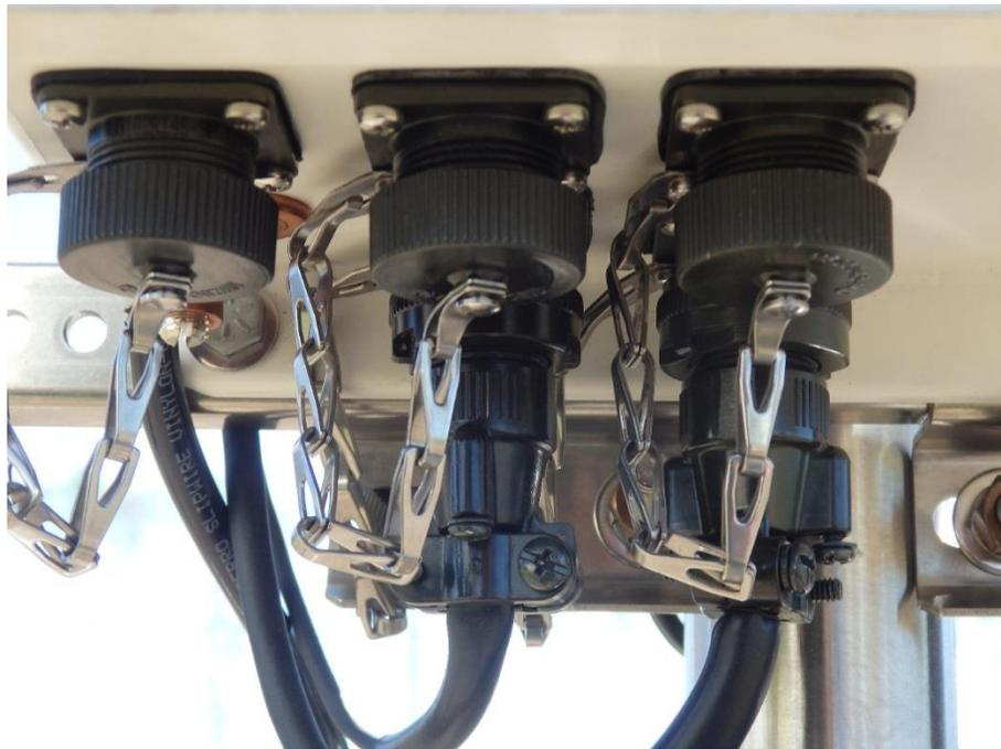
FIGURE 3-10. MET200 Mil-spec connectors
