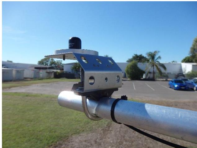
*FIGURE 3-8. Installed SP-212 Pyranometer*
