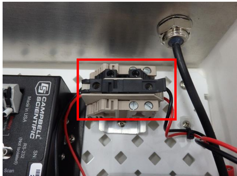
FIGURE 4-3. In-line power fuse needs to be connected for system to Power
