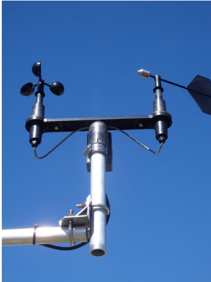
FIGURE 3-7. Installed 03002 Wind Sentry
