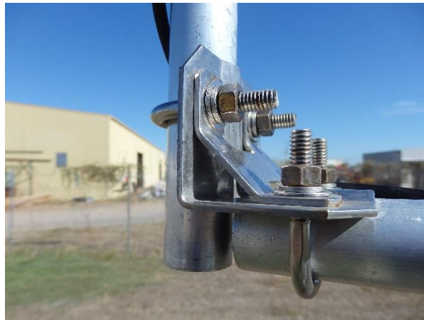
FIGURE 3-6. CM220 right angle bracket used to attach 03002 Wind Sentry vertical mounting pipe to the 1.2m CM204 horizontal cross-arm.
