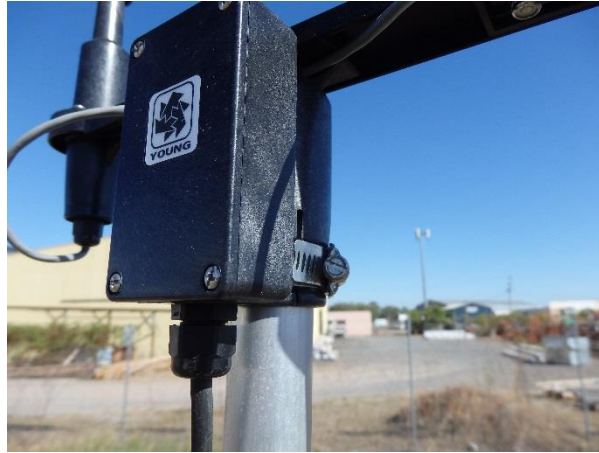
FIGURE 3-5. 03002 Wind Sentry attached to supplied mounting pipe via hose clamp.
