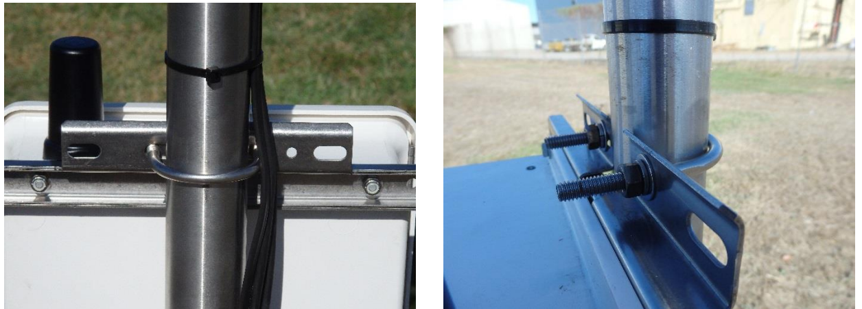
FIGURE 3-2. Mounting the MET200 System Enclosure to a vertical pole
