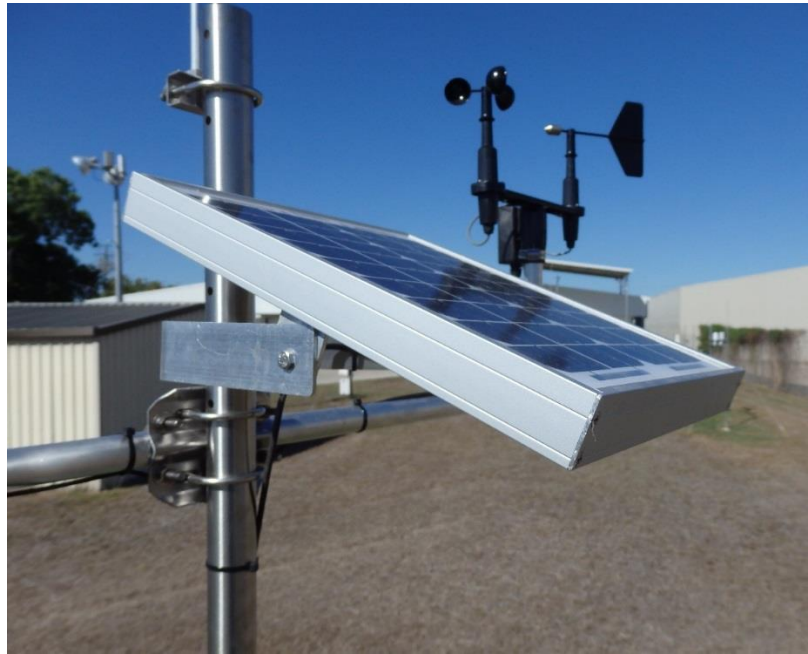
FIGURE 4-1. 10W solar panel and mounting bracket attached to a vertical mast
