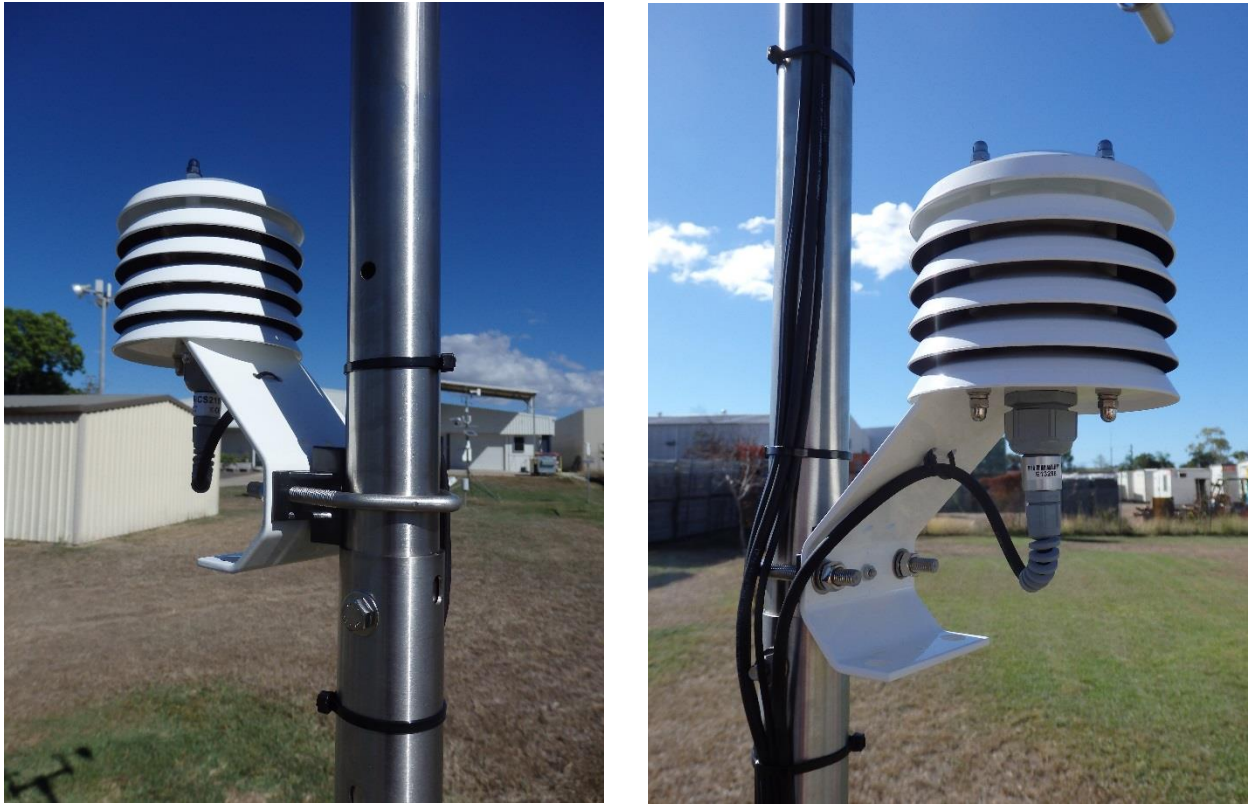
FIGURE 3-4. CS215-MET2 mounted on a tripod mast
