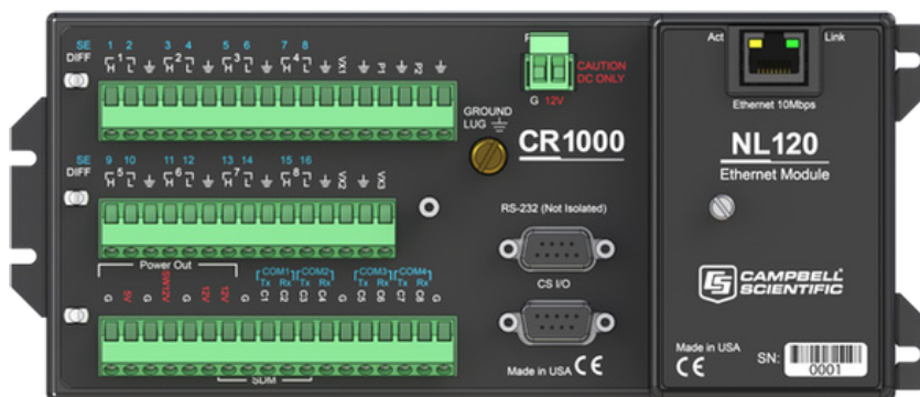
FIGURE 4-1. NL120 attached to a CR1000
